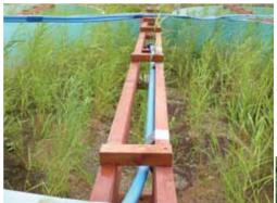
considered are a mechanical centrifugal solution and sludge treatment reed beds. A trial system was required to determine if ferric sludges are suitable for further treatment in Sludge Treatment Reed Beds. The proposed use of reed bed systems reduces the capital and operating cost and provides the site with an environmentally friendly operation area.
